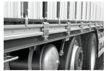
Rails: impact-resistant, galvanised
