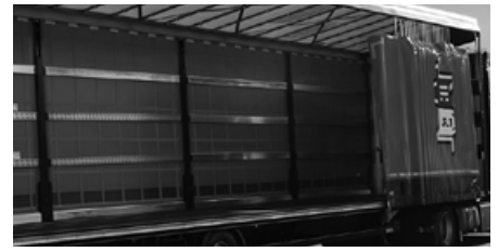
Extended internal width due to tarpaulin
