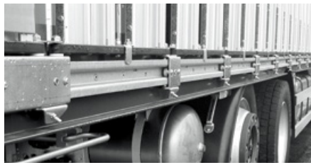
Rails: impact-resistant, galvanised
