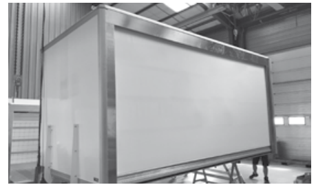
Light aluminium frame for reduced unladen weight
